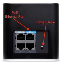
4) Once you have been notified that your service has been activated and subsequently experience problems with connectivity, please try to reboot the AirCube before calling for additional assistance. Rebooting may be accomplished by unplugging the round connector shown in the above picture (power cable) for 30 seconds, then plugging the power cable back into the AirCube unit.
